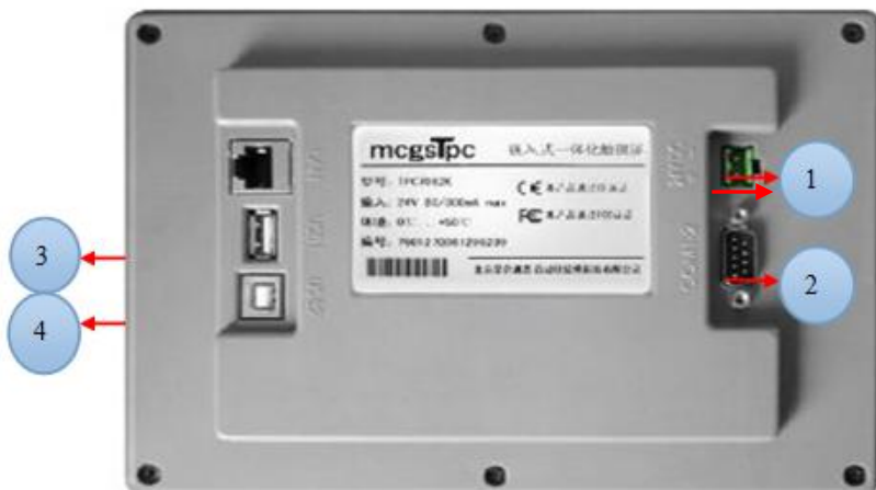
Figure 5-2 Rear View of the User Interface Common port on the back of the display
